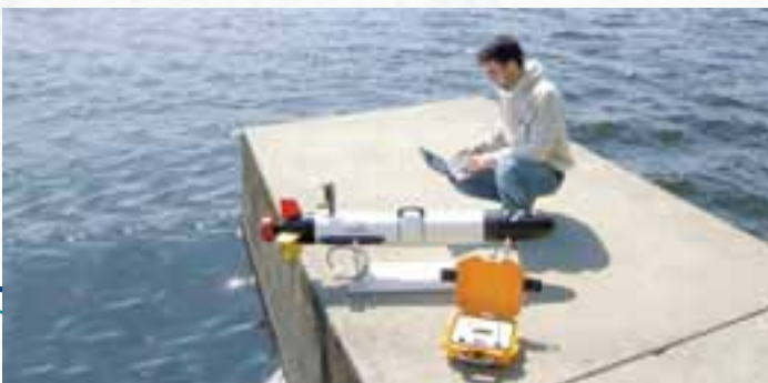
Below: Lightweight and easy to use, Iver2 AUV system can be launched and recovered by a single person
